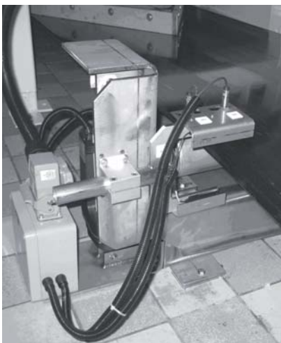
Installation of bernmatic® BTRV Belt Tracking Roller
